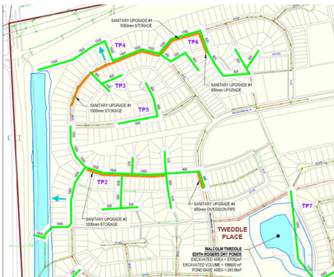
Image 4: Summary Figure highlighting the storm and sanitary system and dry pond upgrades in Tweddle Place.
