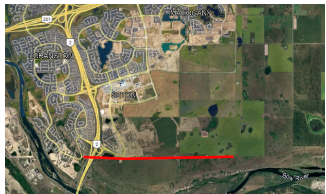
3.5km long, 1.8m internal diameter
