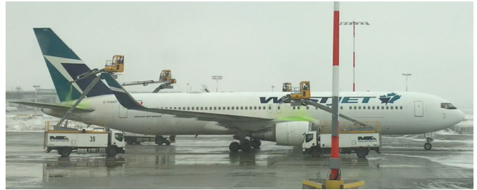
Type I (Green) Aircraft Deicing Fluid Applied on Aircraft
