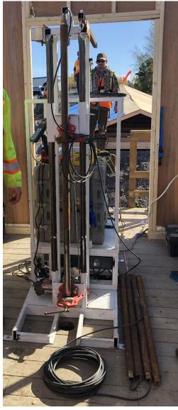
Laser Induced Fluorescence and Electric Conductivity instrument installed and operated from a barge.
