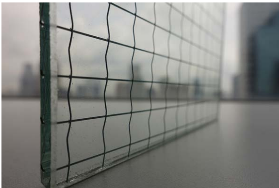
Wired glass should not be mistaken for safety glass.
