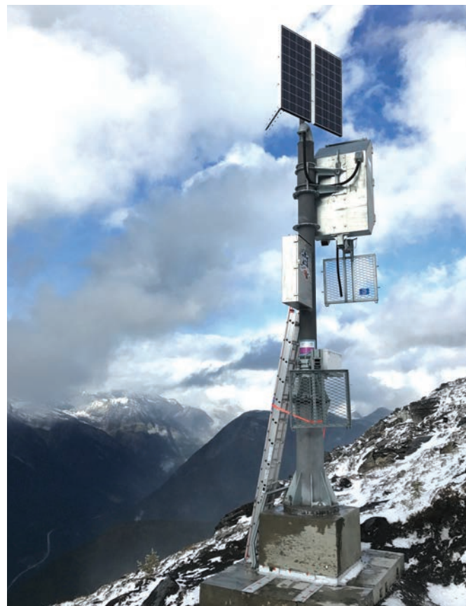
This RACS is solar-powered and its explosives are biodegradable.
