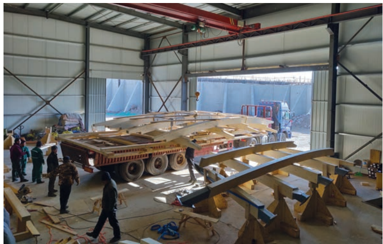
The glulam lattice panels were prefabricated with half-lap scarf joints.
