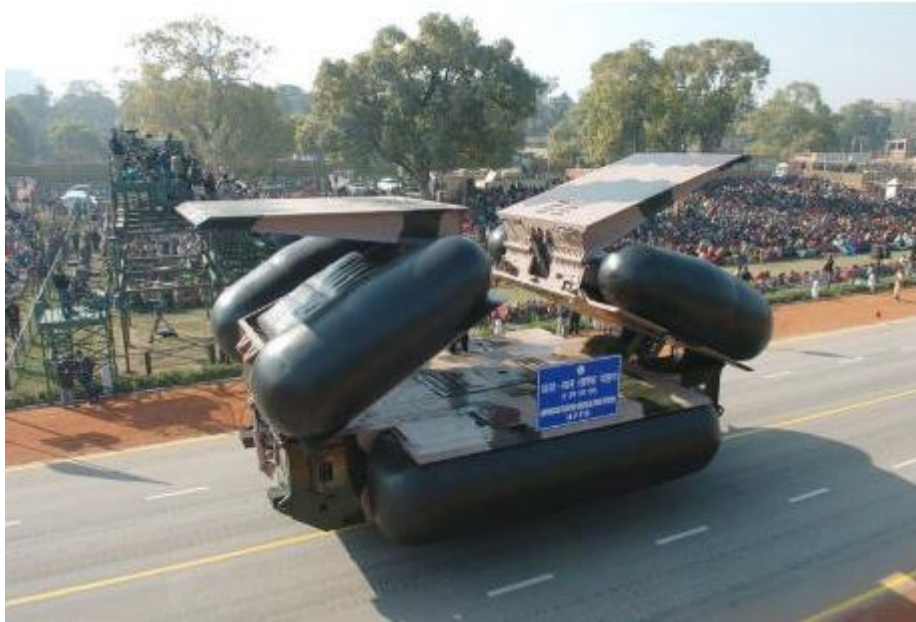
Figure 22: An amphibious mobile bridge system [32].
