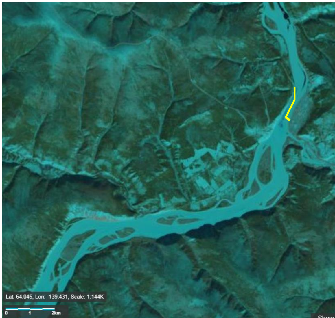
Figure 6: The Yukon River, March 30 2014 (Landsat). Dark narrows bands in the river are open water. That year, an alternative route (yellow line, upper right) for the bridge was necessary, because the ice conditions did not allow it to be built at the usual location [1, 3].
