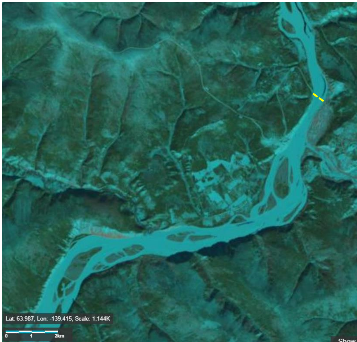
Figure 3: The Yukon River, April 12 2018 (Landsat). The ice cover is light blue. Dark narrow bands in the river are open water. Because these formed at the bridge location, indicated with a yellow dotted line (upper right), that bridge could not be built that winter (2017-2018).
