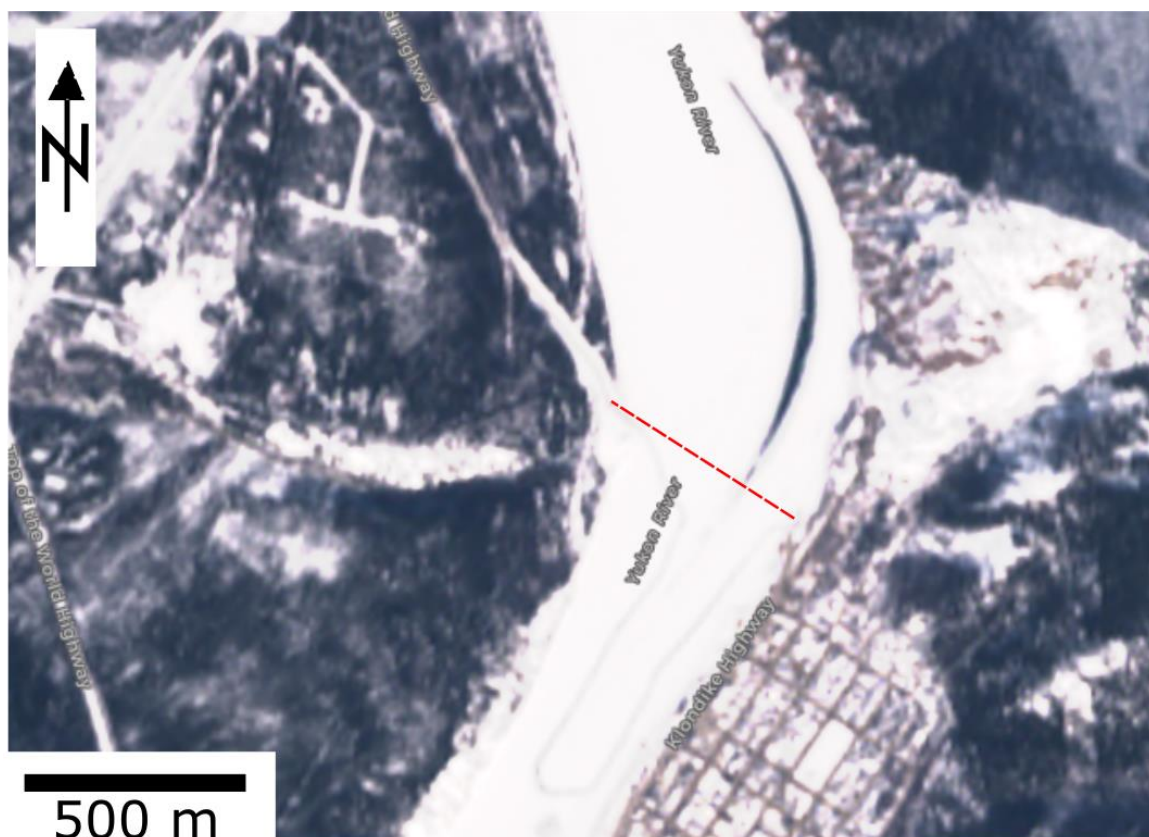
Figure 2: Satellite image of the Yukon River ice cover at Dawson City, April 9 2018 (ESA Sentinel-2). 5 River flow is northward. The dashed red line is where the bridge is usually located – that winter, however, there was no sanctioned ice bridge.
