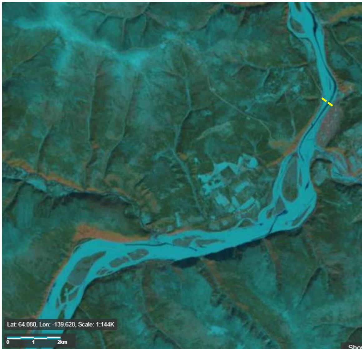
Figure 4: The Yukon River, April 16 2017 (Landsat). Dark narrows bands in the river are open water. The ice bridge was not built that winter (2016-2017) – its usual location is indicated with a yellow dotted line (upper right).
