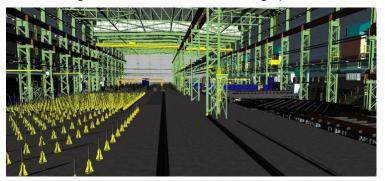
designed, reviewed, analyzed and shared exclusively in Revit with ISI, subconsultants and stakeholders. The implementation of 3D modelling allowed a level design detail and clash detection that was critical to the successful design of this complex facility. This level of detail would have been impossible to achieve using a conventional 2D approach. In addition
