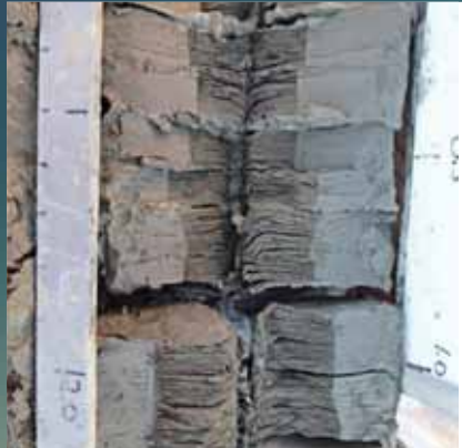
Undisturbed UGLU clay outside failed dam area
