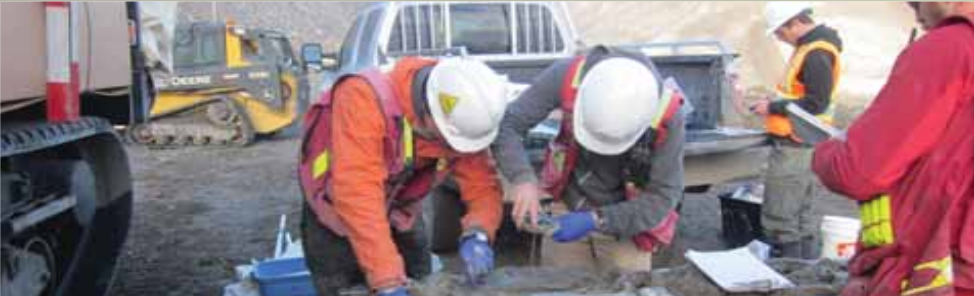
Field examination of sonic drill core
