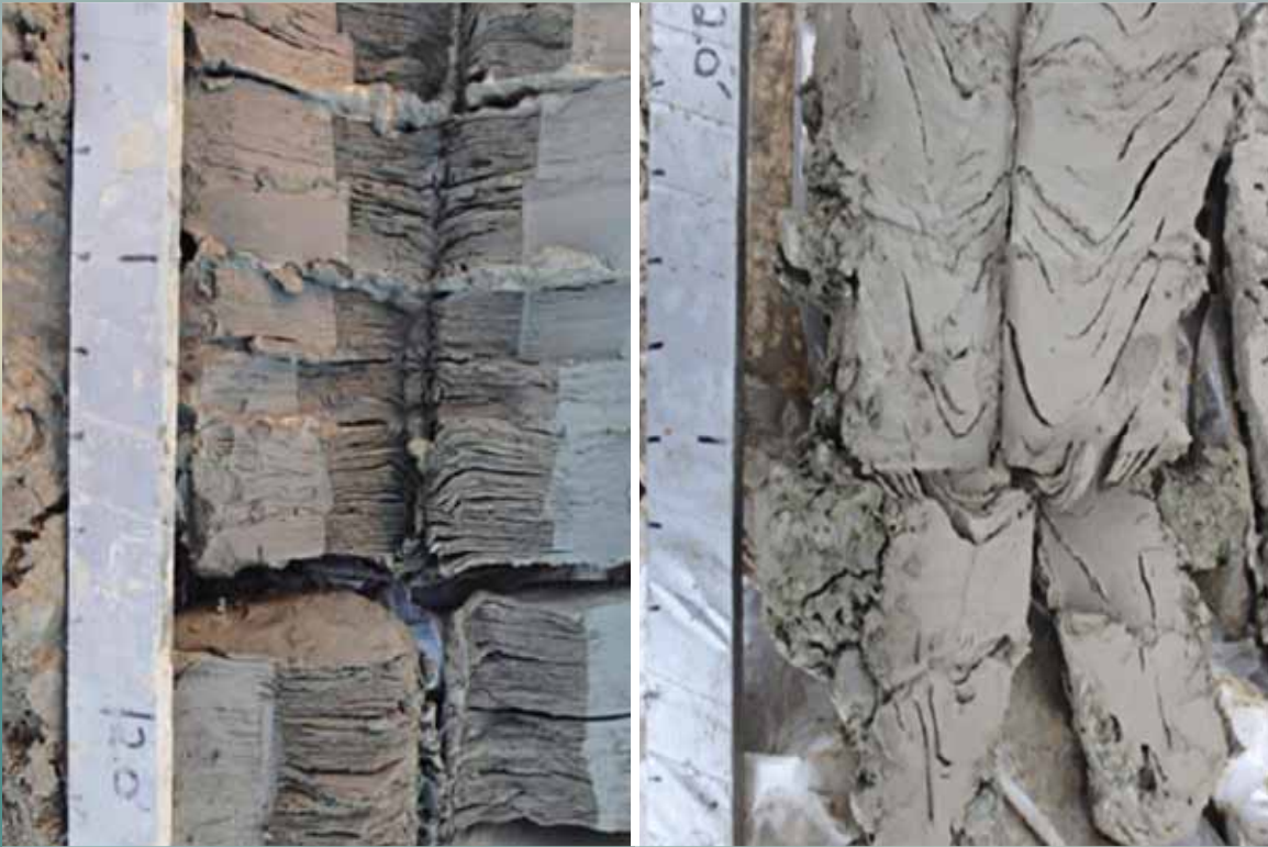
UNDISTURBED UGLU CLAY OUTSIDE FAILED DAM AREA (LEFT) AND DISTURBED UGLU CLAY BELOW FAILED DAM (RIGHT)
