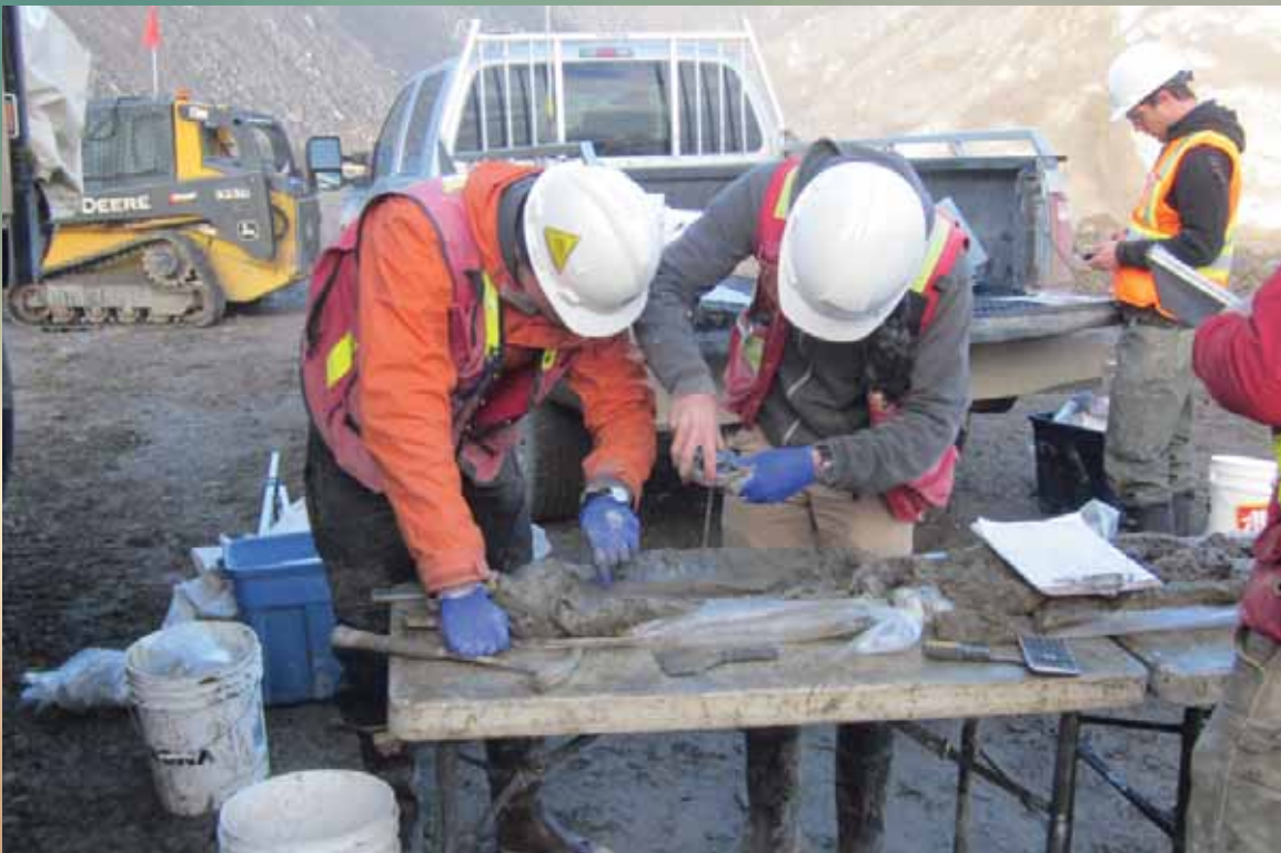
FIELD EXAMINATION OF SONIC DRILL CORE
