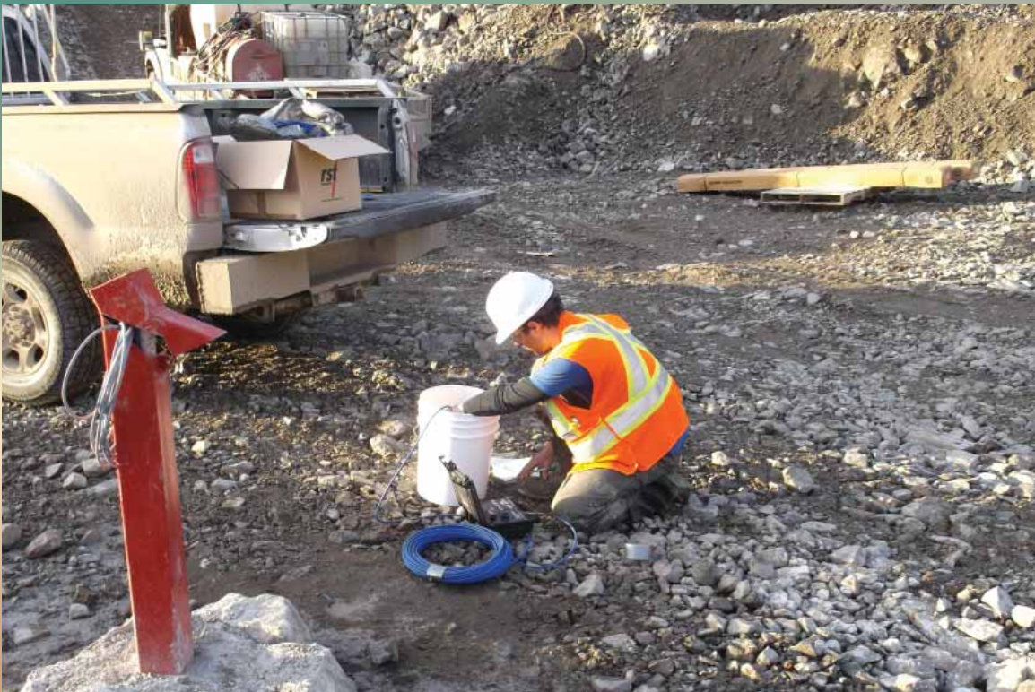
RECORDING OF INSTALLED VIBRATING WIRE PIEZOMETERS
