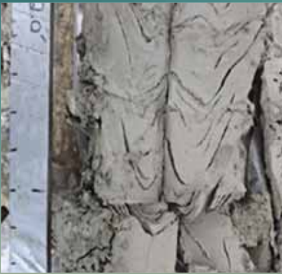
Disturbed UGLU clay below failed dam
