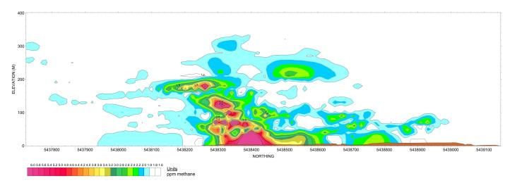
Photo 6 - Contour map of methane concentrations (parts per million) in cross-section through the emission plume downwind (east) of Phase 3 of the Landfill.
