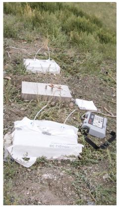
Photo 3 - Flux chamber method measurement equipment. The boxes have a very small footprint area of 0.2 sq.m. compared with the 2,250,000 sq.m. area of the Landfill.
