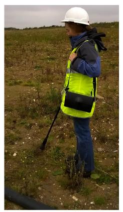
Photo 2 - Conducting surface emissions monitoring. This method measures only atmospheric concentrations of methane and does not measure methane emission rates.
