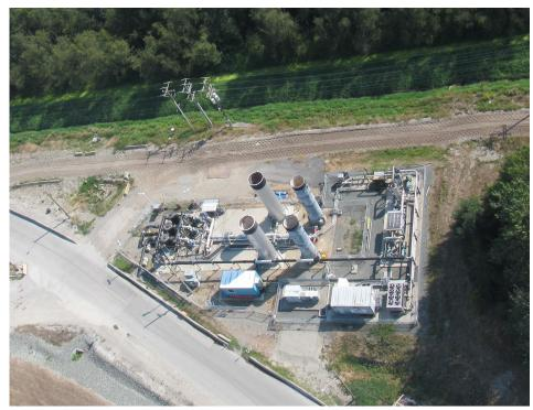
Photo 9 - AMM method measurements can be used to identify the most cost effective method for reducing GHG emissions, thereby maximizing the landfill gas that is utilized, or combusted in these flares.
