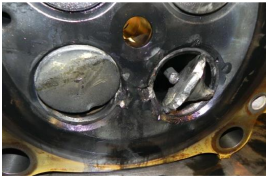
Broken intake and exhaust valves
