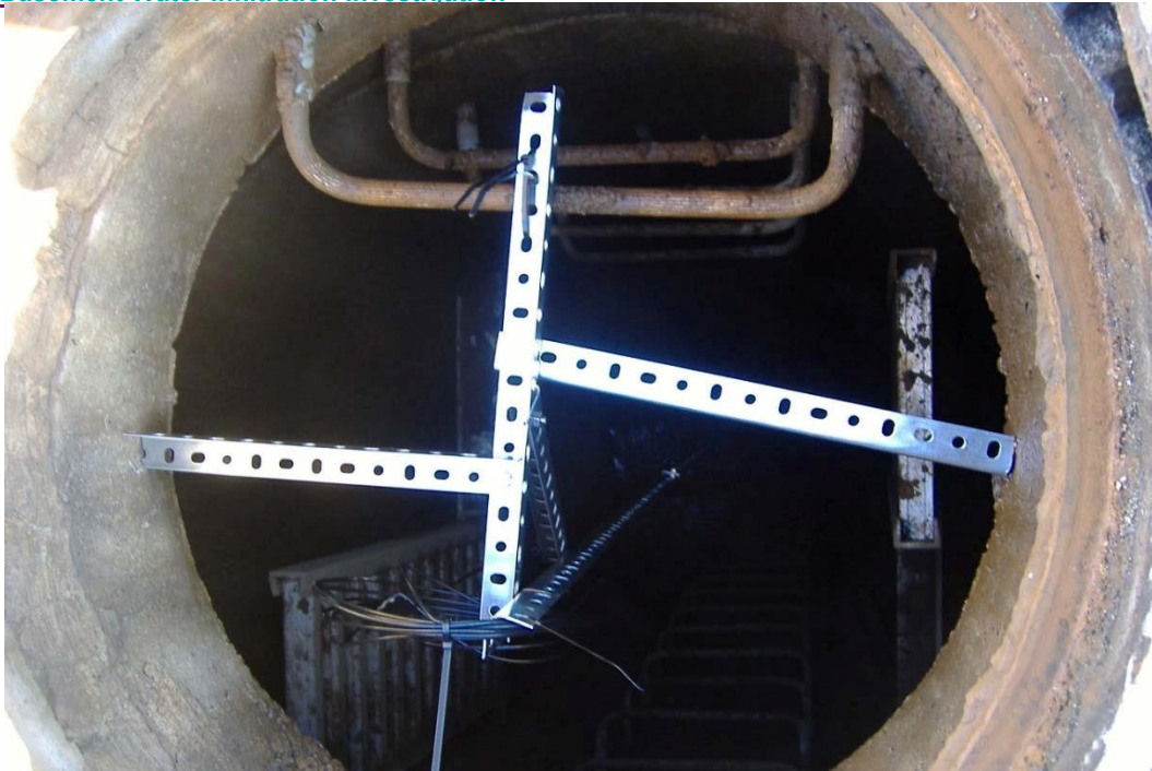
Top View of Typical FDC/Storm Sewer Maintenance Hole Gauge Installation
