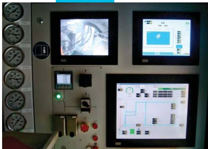
MTBM controls, tunneling operator displays
