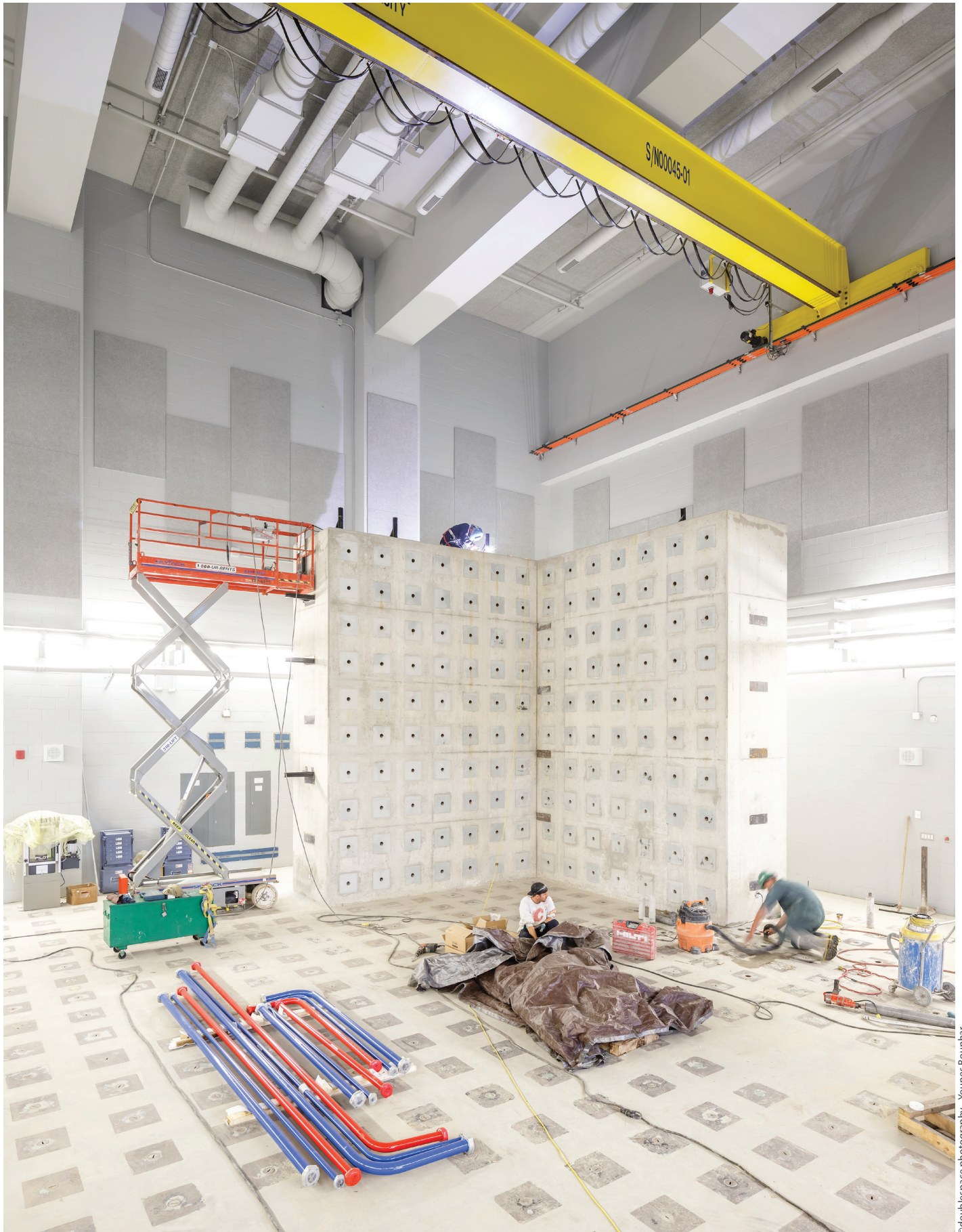
Three-storey civil lab with strong wall and floor.
