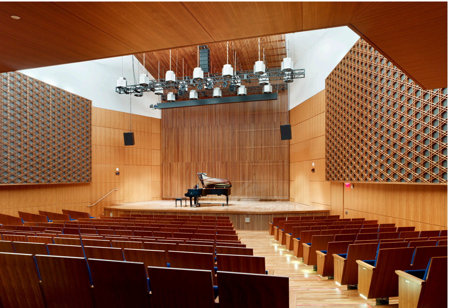
Aga Khan Museum Auditorium: The HVAC displacement system, controlled from grilles hidden beneath each individual seat, is barely visible.
