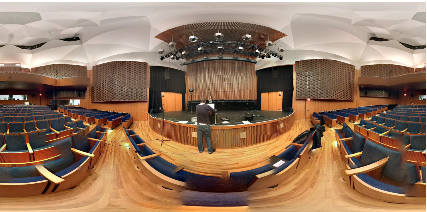
Aeroustics staff on site at the Auditorium conducting WinMLS measurements. The single omnidirectional dodecahedron (12 sided) loudspeaker is visible on stage.
