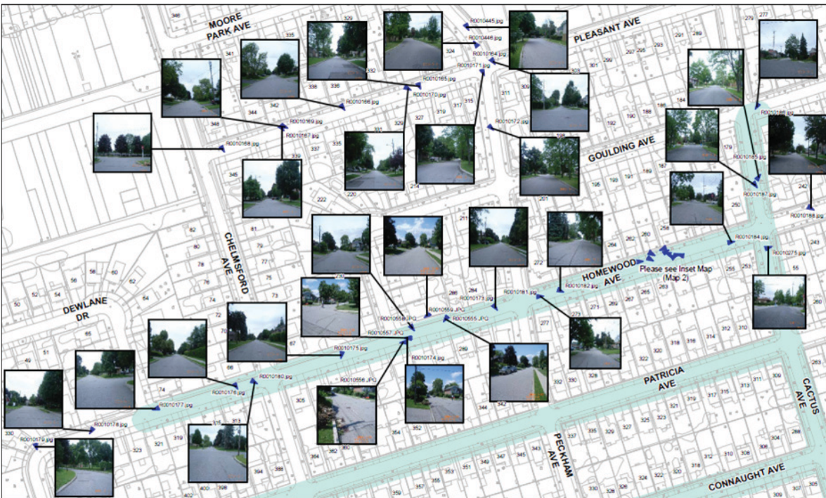
GPS-Enabled Camera for Site Photographs: Hundreds of site photographs are automatically logged and organized to assist with construction inspections.
