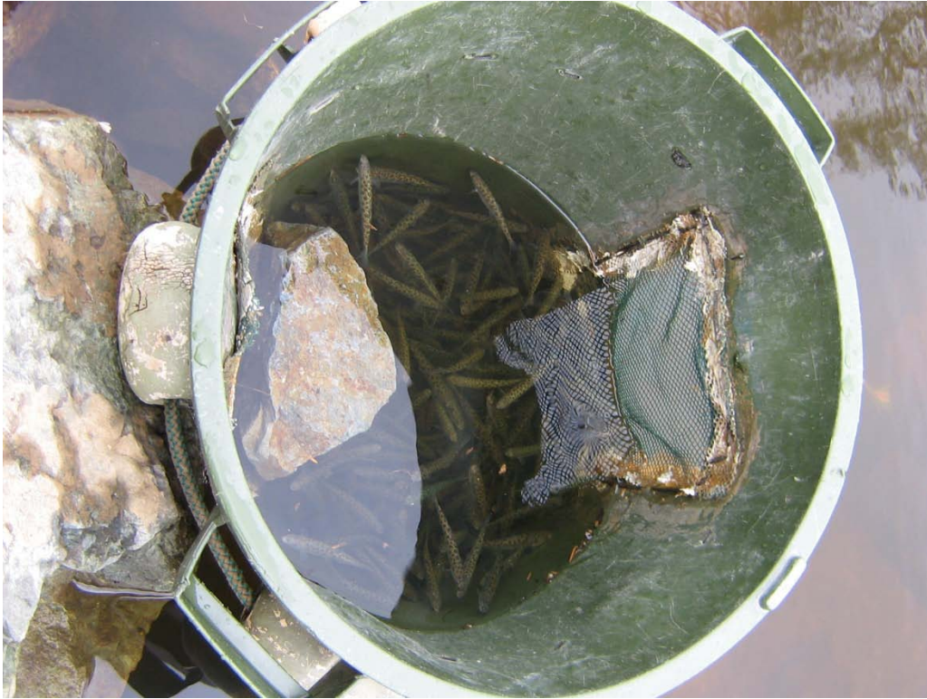
Hatchery Chinook and Coho Salmon used for live fish testing. Ninety percent of transferred fish passed without harm.
