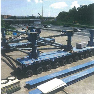
Assembled Self Propelled Modular Transporter (SPMT) stationed in the staging area
