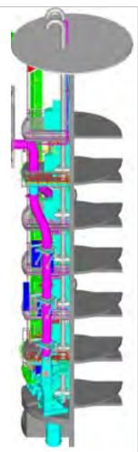
3D model view of the Micro-Hydro and Baffle Drop sides of the WWTP shaft
