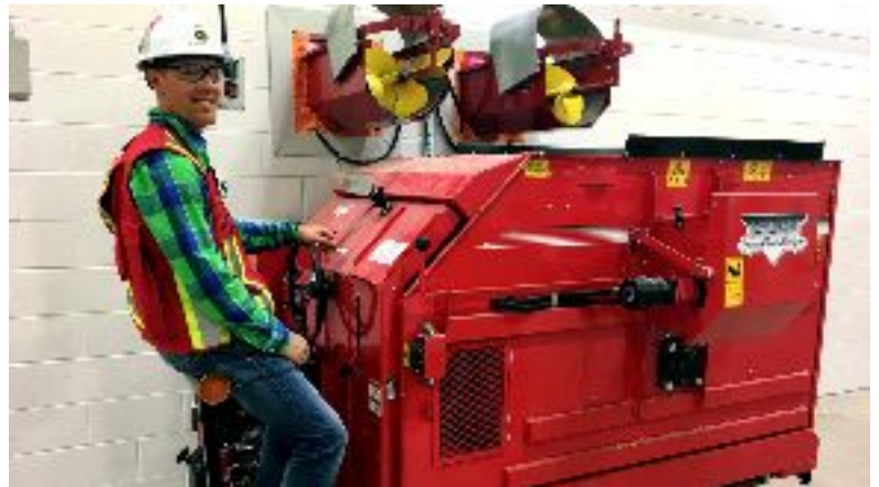
The Data Ranger automated feed mixer and dispenser system helps researchers monitor food intakes for the intensive feeding trials
