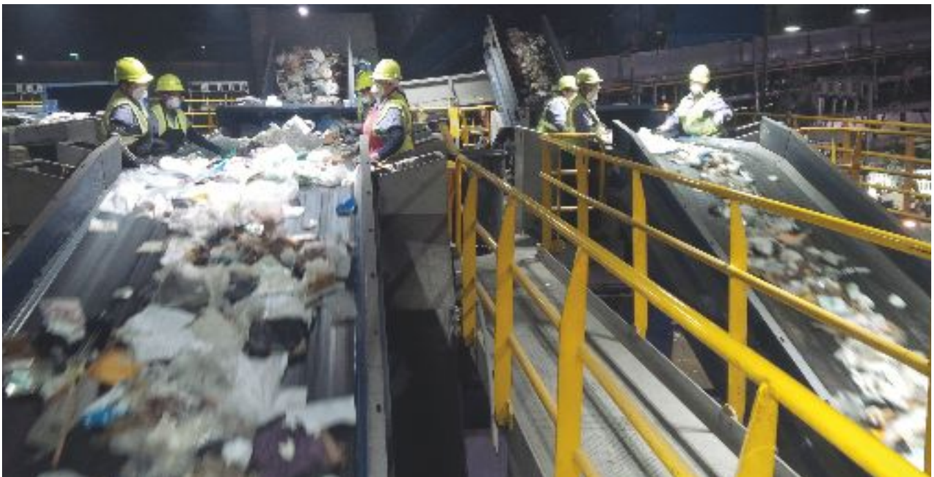
Hand sort station to maximize recovery
