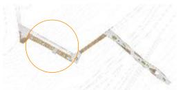
The stairs are supported on galvanized steel stringers. These light weight components simplified erection and assembly. Construction access was limited with lift points only at the top and bottom of the stairs because of the steep slope. The stair stringers have varying geometrical and loading requirements to accommodate the architectural aesthetic and varying urban stair geometry.
