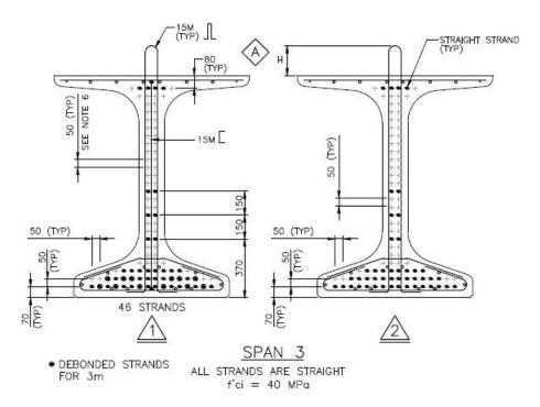
It is very important for the economical production of precast and prestressed components that the designer specifies the minimum concrete strength at transfer, (f'ci), rounded to the nearest MPa, which the Code SLS requirements will permit. Specifying the minimum concrete strength required ensured that the girders can be poured, cured and stripped on a 24-hour cycle.
