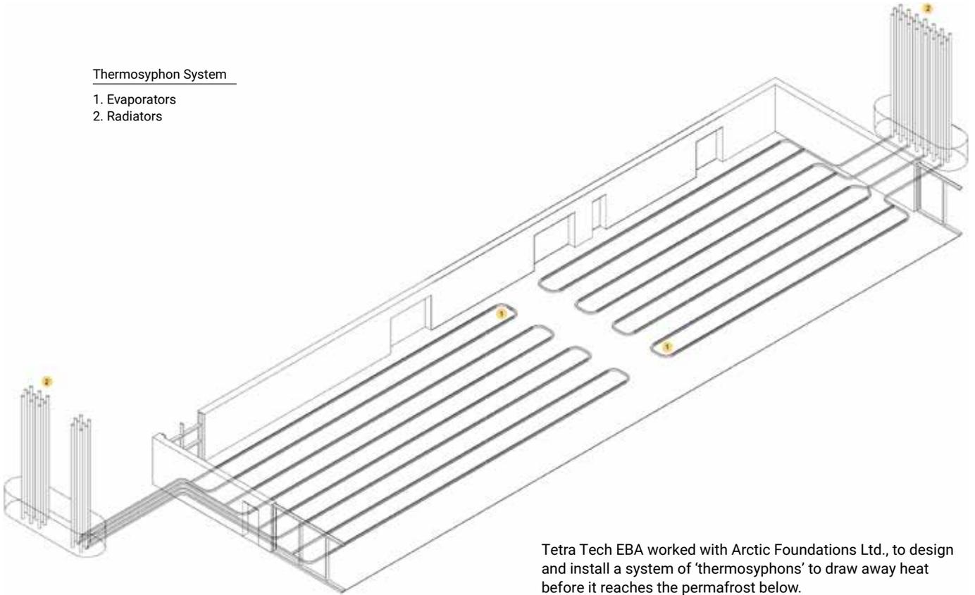
Tetra Tech EBA worked with Arctic Foundations Ltd., to design and install a system of 'thermosyphons' to draw away heat before it reaches the permafrost below.
