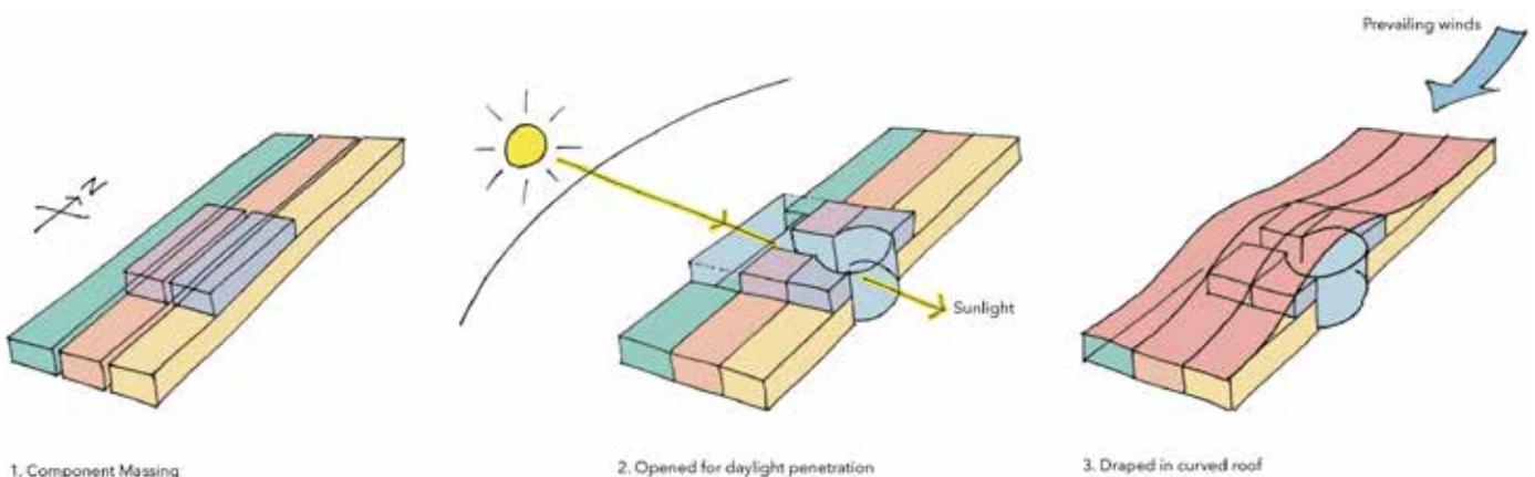
A simple rectangle design minimizes the number of building corners, and the sinuous curving roof minimizes surface area of the building envelope, providing a smooth surface for winds to scour the roof free of drifting snow.
