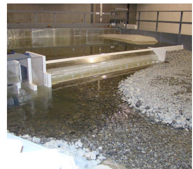
Headworks, physical hydraulic model, 1:12 scale
