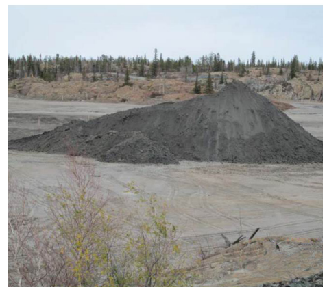
Photo 11 - Stockpile of Processed Tailings for Paste Production
