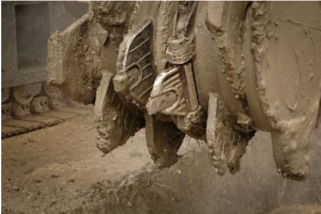
Image 11: BCM10 cutter head mixing wheels fitted with TungStud cutting teeth
