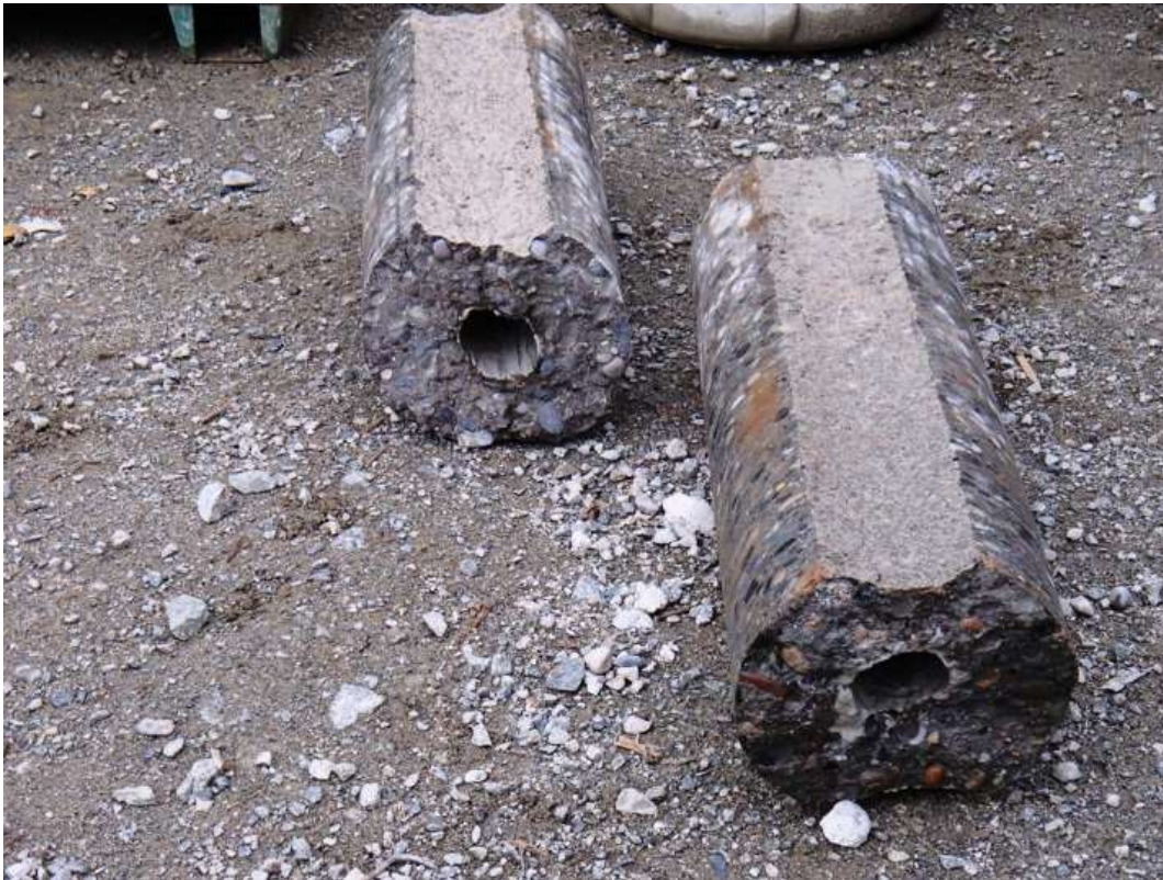
Image 2: Cores from secondary location showing inverted pendulum pilot hole
