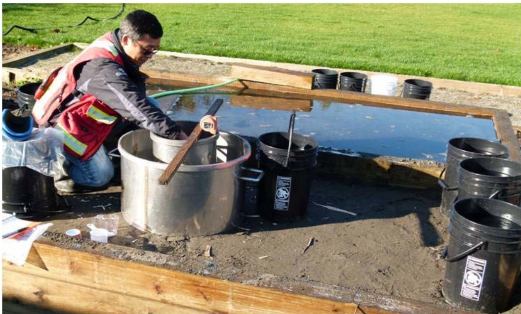
Photo 4 – Pilot Testing Soil Filter Media Bed
