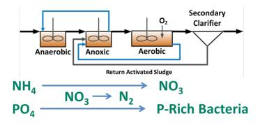
Figure 1: Illustrating conventional secondary treatment with the primary function of converting soluble organic contaminants into bacteria and converting ammonia to nitrate.
