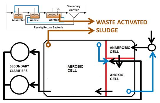
Figure 4: Illustrating the three cell BNR configuration and recirculation for a conventional mechanical process (upper left) and the parallel configuration and recirculation within the modified Kamloops lagoon process.
