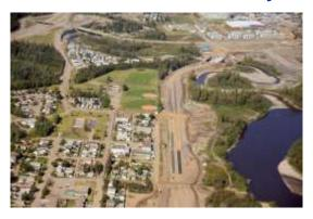
Design and construction of the Gregoire Sanitary Sewer project in Fort McMurray posed significant risks and challenges. The continuous, 1.6 kilometre, 600 millimetre diameter, dual sanitary sewer system traversed a business area, soccer field, children's play park, a busy roadway, and Highway 63—a major highway and the only transportation link to the oil sands development north of Fort McMurray. The sewer alignment included significant environmental and geological constraints.
