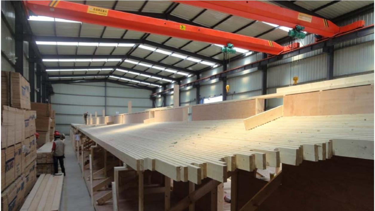
Figure 1: The team developed a design idea that could be simply constructed on site in China – a warping wood plate that consisted of straight pieces of ordinary Canadian lumber and plywood, fabricated into panels in a temporary shop on site with the aid detailed drawings. Photo Credit: StructureCraft Builders
