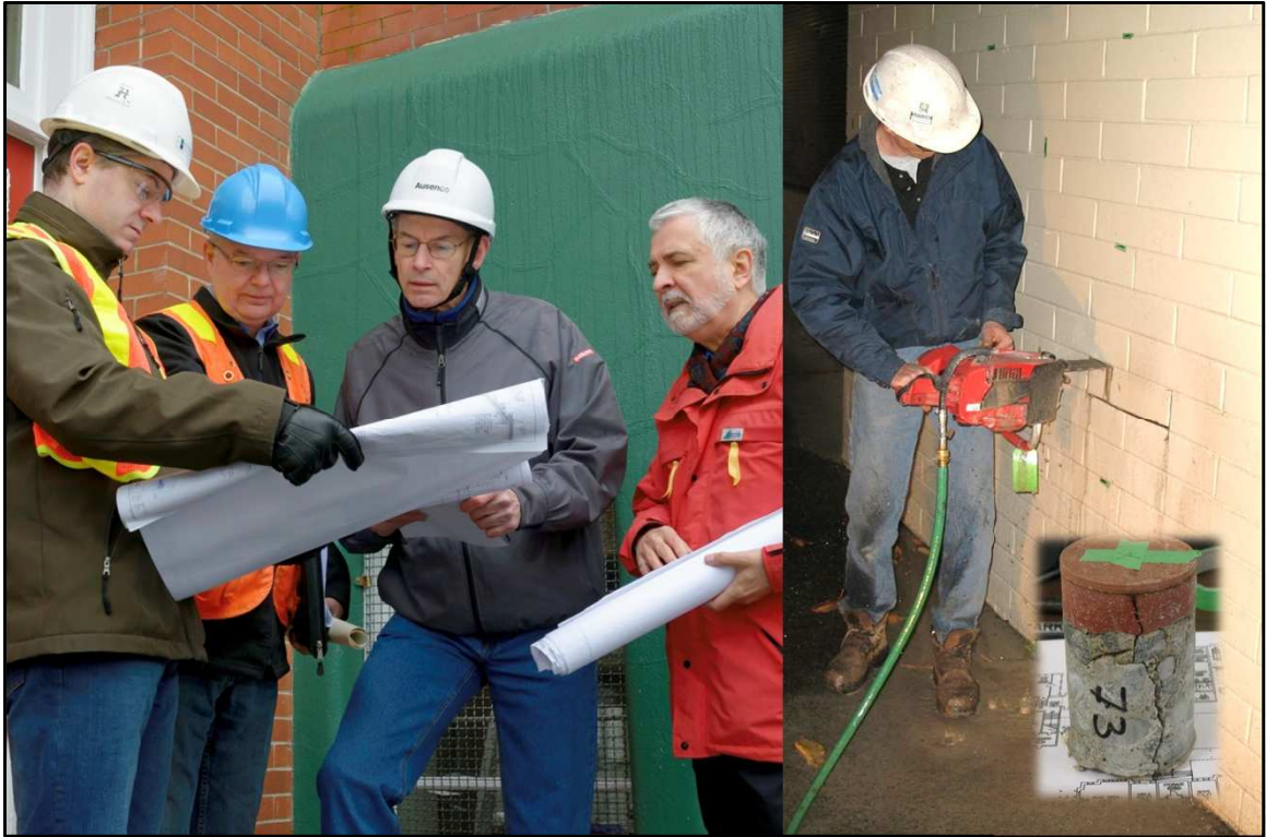
Site inspection and review of drawings to determine existing structural “prototypes”, coupled with material testing to enable calculation of their seismic capacity.
