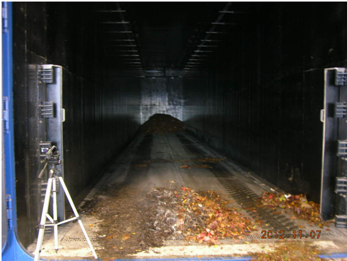
Figure 4 First Filling of Organic Waste into a Percolator
