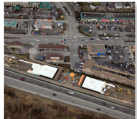
January 26, 2011 - Aerial looking north. Westbound lanes under construction including EPS approach fills and pier caps. All traffic detoured to south side of right of way.
