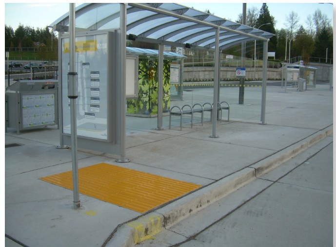
April 2013 - One of the two large bus shelters (open face concept for Vancouver weather) with new power distribution box for entire site behind at Carvolth Exchange. Tactile yellow handicap pad in foreground, new retaining wall and Park and Ride in background.
