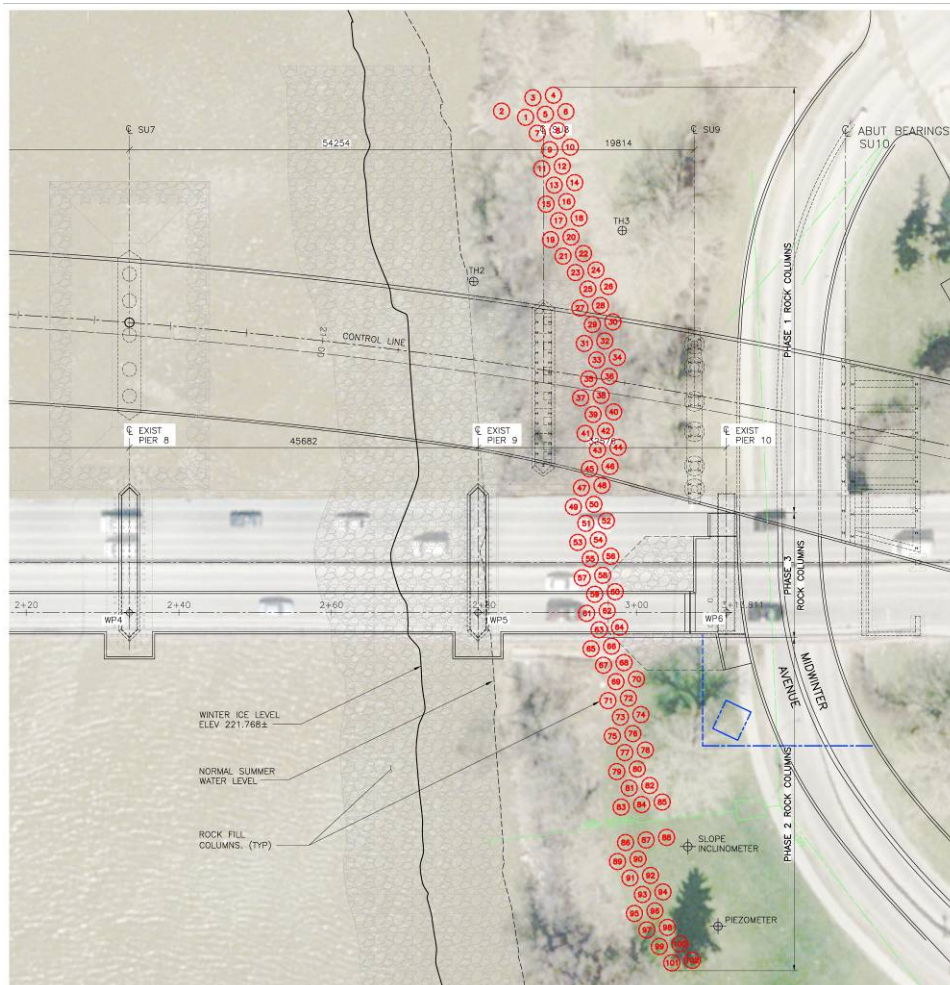
Figure 4 – River Bank Slope Stabilization
