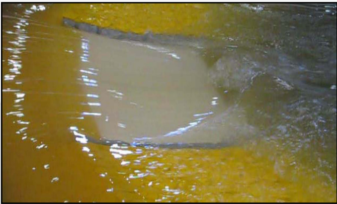
HWC Drop #3R flume model
