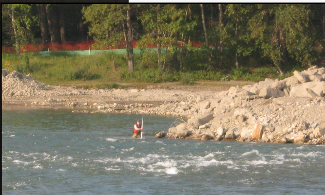
Velocity measurements in river diversion
