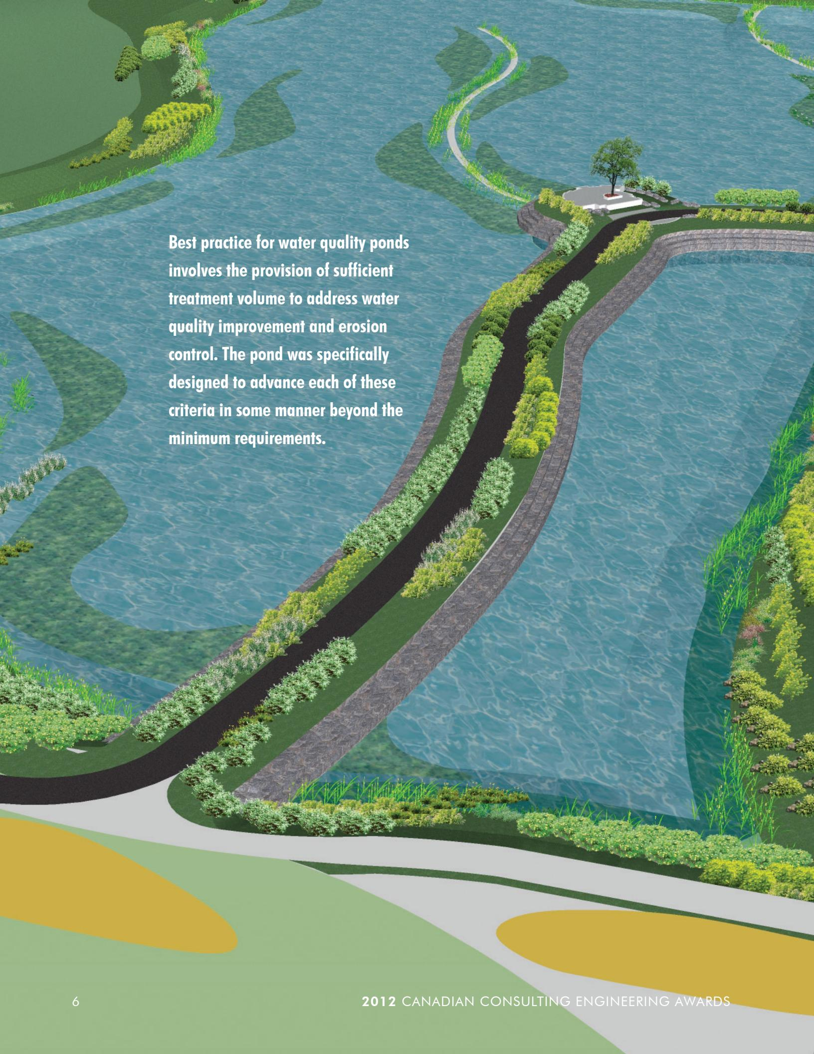
**Best practice for water quality ponds involves the provision of sufficient treatment volume to address water quality improvement and erosion control. The pond was specifically designed to advance each of these criteria in some manner beyond the minimum requirements.**
