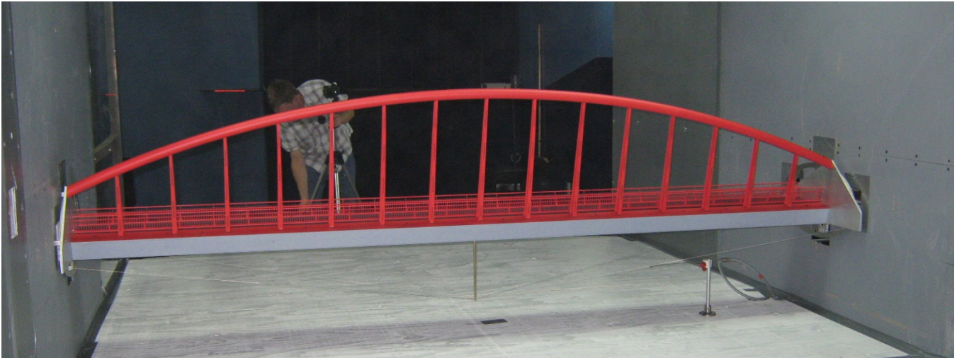
Figure 11: Wind Tunnel Testing
