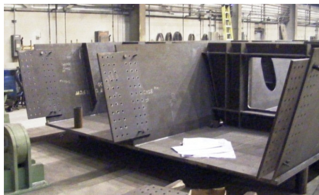
Figure 8: Fabrication of Trapezoidal Steel Box Girder
