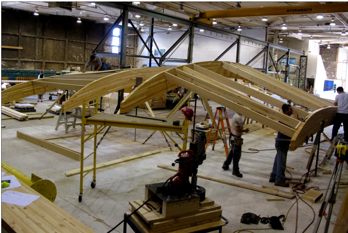
Figure 6 – Prefabrication at the shop, using glue-laminated beams as a jig to frame the complex geometry.
