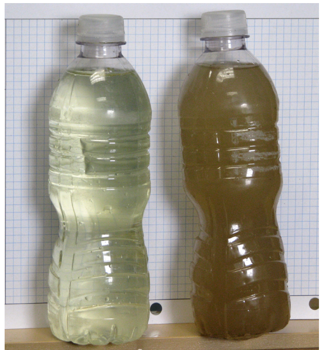
Treated Water (Left) from the Former Water Treatment Plant and Raw Source Water (Right) from Sousa Creek (April 2010)
