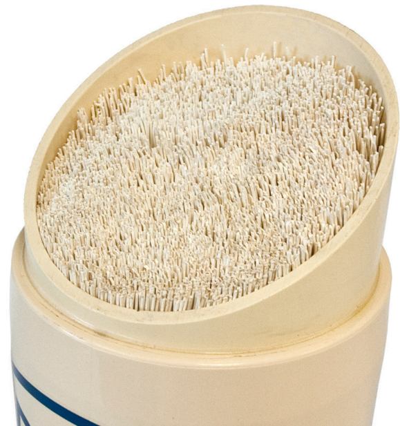
Close-up of Microfiltration Membrane Cut-off
