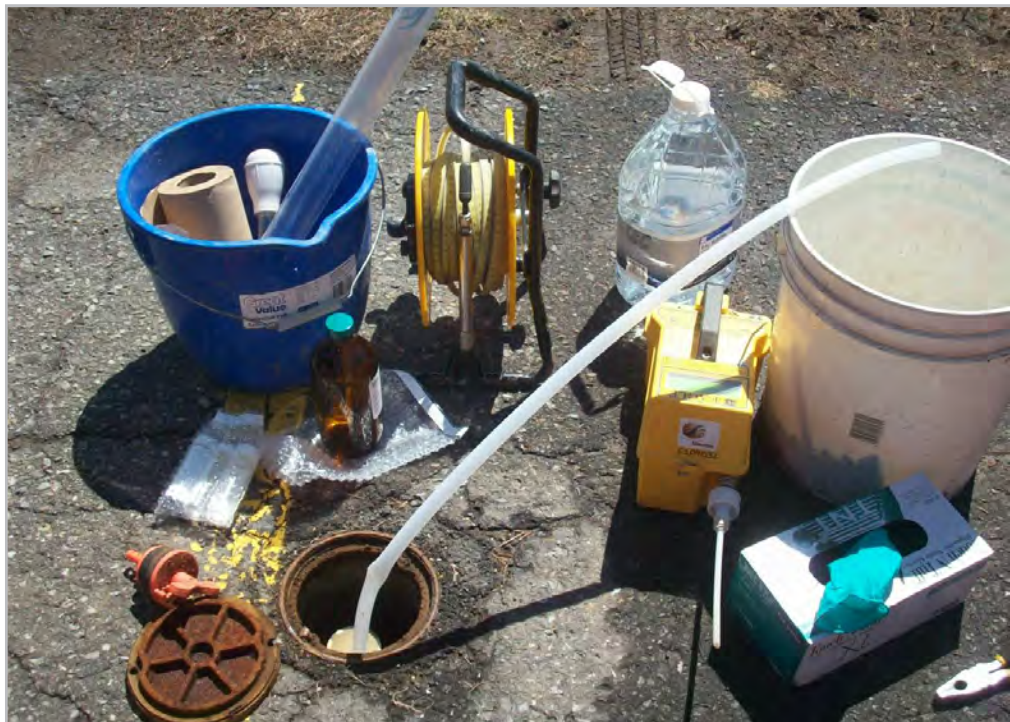
Groundwater sampling at the Booth Street Complex
