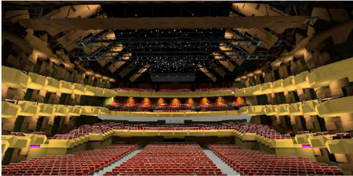
Figure 2. Computer rendering of the 2nd renovation design. Note the ceiling reflectors, inspired by Christchurch Town Hall and the narrowing of the orchestra level at the back, inspired by the Vineyard Step layout of Berlin Philharmonie.
